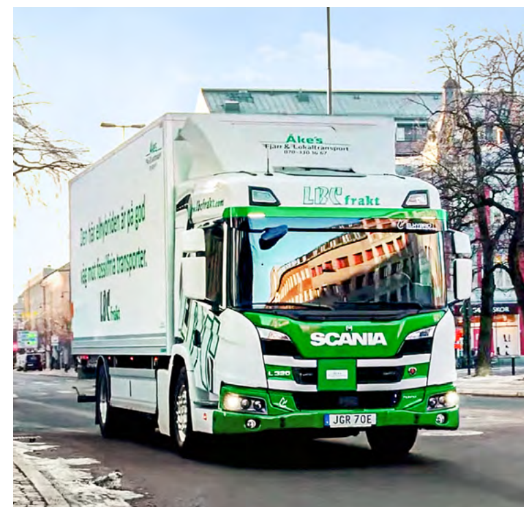
Clean delivery: Swedish company LBC Frakt AB is relying on a Scania plug-in hybrid truck for its transition to fossil-free transports. The truck runs on electricity supplied by the company's own solar system or on organic diesel.
