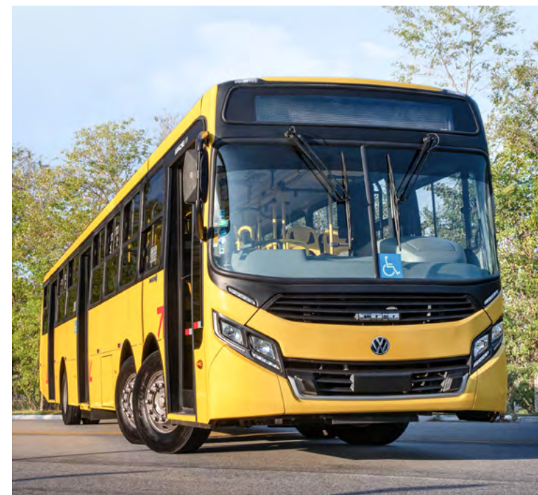
A bus with extra length: the new model from Volkswagen Caminhões e Ônibus is being tested in Brazil. With a length of 15 meters, this super-bus can accommodate up to 115 passengers.
